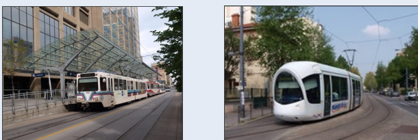
Edmonton's "suburban" high-floor LRT vehicles (left) will be replaced with new "urban" low-floor vehicles, as shown at right.
